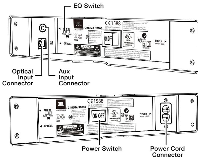
**EQ switch:** Use this switch to adjust the soundbar's bass for either wall or table mounting. If you're mounting the soundbar on a wall with the included wall-mount bracket, set the EQ switch to the "Wall" position for the most natural-sounding bass performance. If you are placing the soundbar on a table, set the EQ switch to the "Table" position for the most natural-sounding bass performance.
