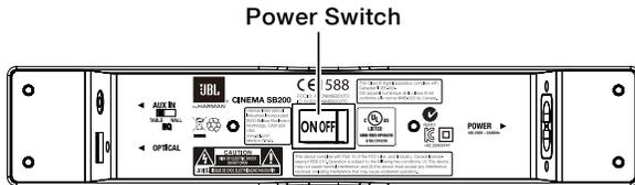
Press the Power button on either the soundbar or the remote to turn the soundbar on. To put the soundbar in the Standby mode, press either Power button while the soundbar is on.
